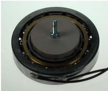
Figure 3. Foto of a rotating ball bearing used in the measurements
