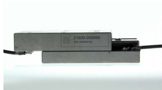
Figure 1. Photo of a linear friction bearing used for the measurements
